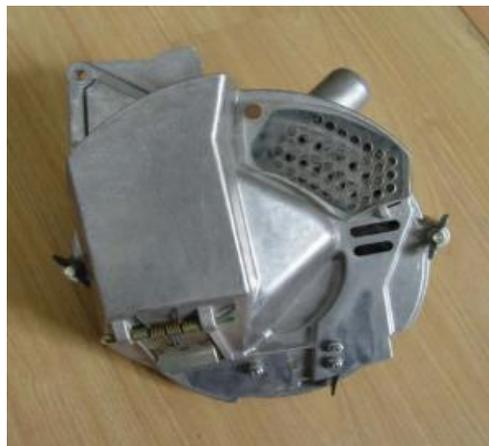
**Figure 3 Suction seed-metering device**
