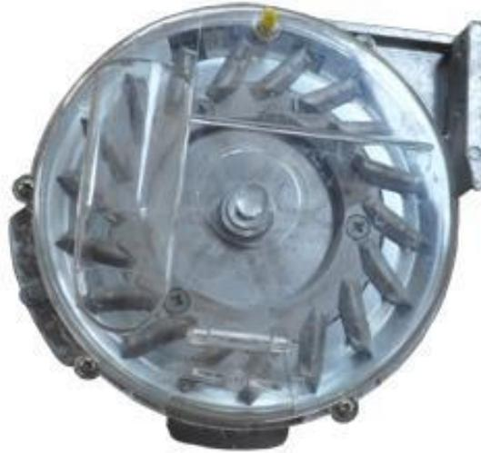
**Figure 2 Spoon type seed-metering device**
